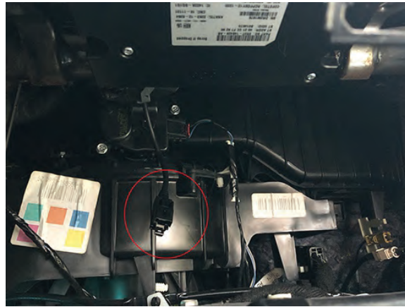
Step 11 (Sync Vehicles Only) Remove the USB cable from the Sync module.
