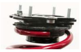
9. Re-Install the strut nut and torque to factory specifications. Spring not shown. (Do Not Use Impact Guns).
