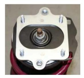
13. We install one 8mm nut onto one of the studs to keep the caster plate in place during shipping. <u>Make</u> sure to remove this nut before trying to install the assembly into the car.
