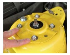
15. Install the supplied M10 x 20mm bolt with 10MM support washer into the caster slot in the factory tower. You can now snug all 5 mounting bolts and nuts.
