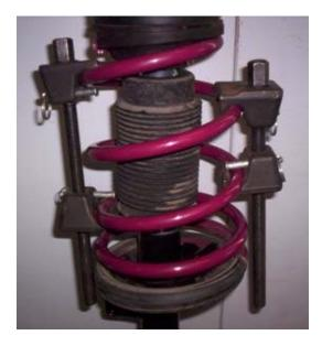
6. The spring is compressed enough when the spring has no pressure on the upper mounting plate, as shown to the right.
