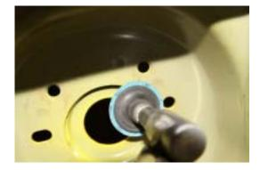
12. The camber plate has a offset bearing design which allows you to install them in a street setting or a race setting. To install in the street setting which will allow you to more positive camber for lowered cars simply install with the notch toward the inside of the car (engine side) and the race setting you will install the notch toward the fender (outside) of the car.
