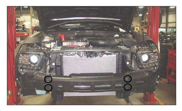
4. With a 13mm socket remove the inner four (4) front bumper reinforcement bolts.
