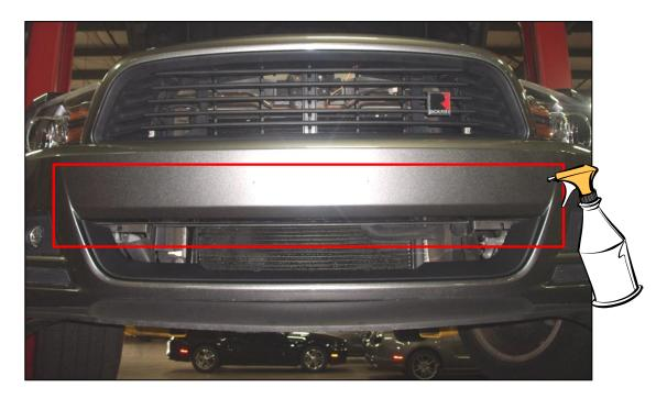
2. Remove the white backing from the black graphic (1313-17K945GR) and apply soapy water to the backside of the graphic to aid in installation.
