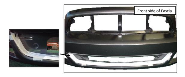
12. Using a china marker or other marking device, mark the two slots cutout at the ends of the templates. Using an automatic center punch, mark the locations of the eight (8) holes on the lower mouth template.
