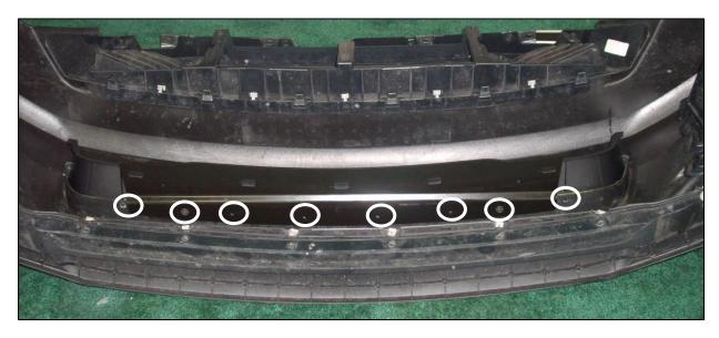
13. Install the seven (7) retaining clips (21067) onto the seven (7) lower mouth trim tabs, centering the tab within the clip and pressing firmly. **Note: a drum brake spring tool is recommended for pressing the clips onto the tabs.**
