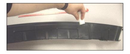
2. Install the tape (1313-17K945TAPE) onto the lower mouth trim piece as shown in the image below.
