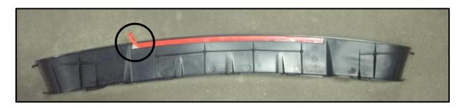
9. Loosely place the lower mouth trim piece into the lower grille opening. Line up the tabs in the left and right corners with the slots of the fascia. Be sure the tape film is accessible for removal.
