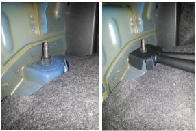
Note: This brace is designed to work as either a bolt-in option or weld-in option. If a weld-in installation is desired, be sure to prep the body surface & brace surface properly before doing so. Bend the tabs of the brace to meet the body of the vehicle before welding. Make sure all welding/finish coating is complete before moving to Step 4.
