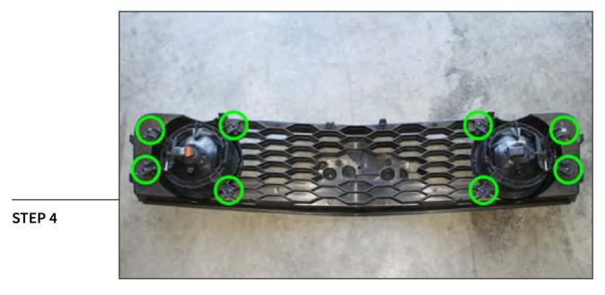
Remove the (8) 7mm screws securing the fog light mounts to the grille. The 05-09 grille shown above, the 10-12 fog lights mount similarly.
