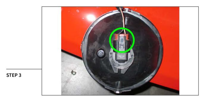
Press down on the electrical connector to release the fog light harness from the fog lights.
