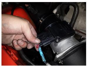
Step 7. Plug in the MAF sensor and IAT sensor using the factory wiring.
