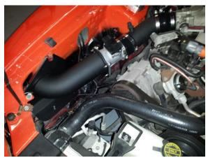
Step 6. Install the lower part of the intake tube onto the upper portion using the supplied coupler as show above and slide it into the shroud.
