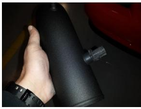
Step 3. Install the IAT sensor into the intake tube as shown.
