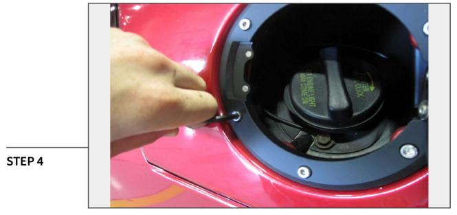
Once the hinge side of the door is secure, tighten the Allen head screws securing the tabs to the rear of the body as shown. This completes the installation of you new Billet Fuel Door.
