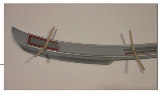
Center all 4 drilling templates over each of the 4 mounting points.
