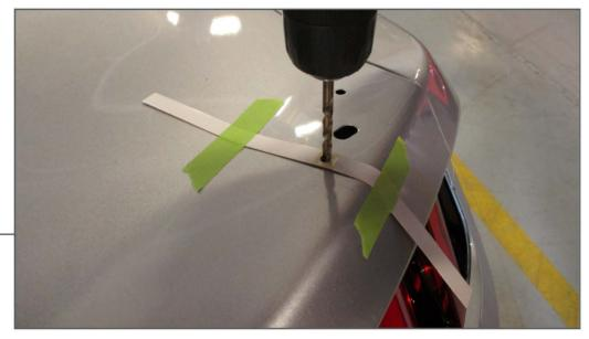
Once the spoiler is removed, carefully drill the center of the template holes. Finish with a 7/32's drill bit. Use clear nail polish to cover any exposed metal to prevent rusting.
