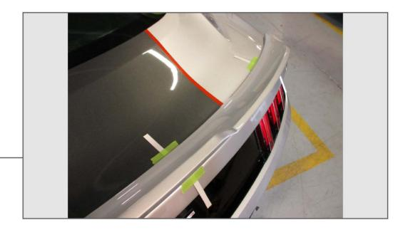
Test fit the spoiler and center it on the decklid. Then tape the templates to the decklid where they lay. Carefully remove the spoiler from the templates. This step is extremely import and will determine the final fitment of the spoiler. Please take your time and ensure the spoiler is seated properly before taping down the drill templates to the decklid.
