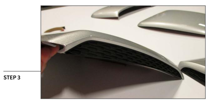
Remove the tape backing from the insert and install in the recessed opening on the front of the scoop. Make sure the top of the insert sits flush against the top of the opening. If the bottom of the insert sticks out past the body of the scoop, it may prevent it from sitting flush on the window.
