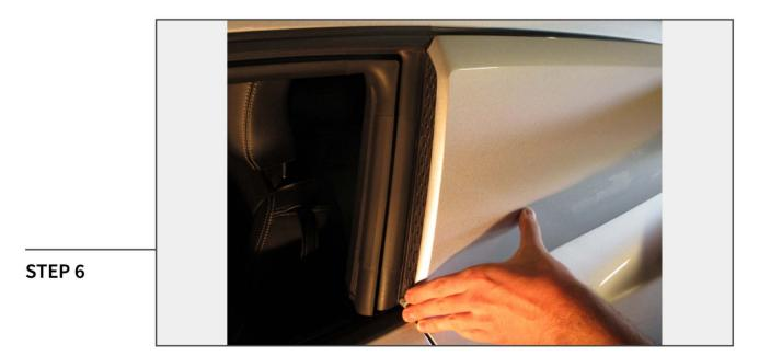
Once the quarter window scoop has bee properly aligned, press down firmly on all taped areas to fully seat the adhesive. Wait at least 24hrs before attempting to separate the scoop from the Dual Lock tape. Repeat these steps for the opposite side.
