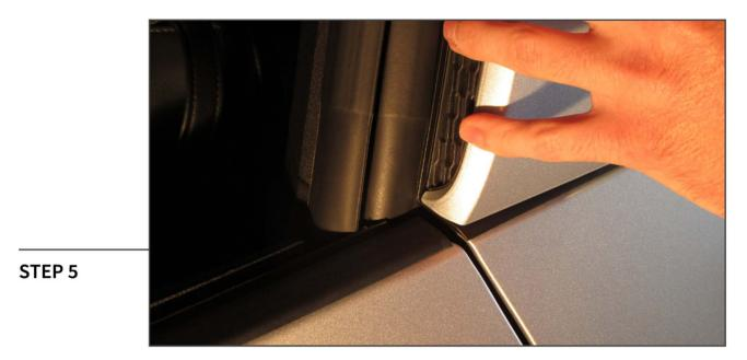
Remove the tape backing. Align the bottom edge with the edge of the quarter window molding. The front edge of the scoop should be parallel with the edge of the window glass. The top edge of the scoop should follow the style line/groove in the quarter window molding.
