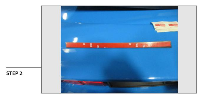
The tape brackets are side specific, the bracket shown is the LH side.
