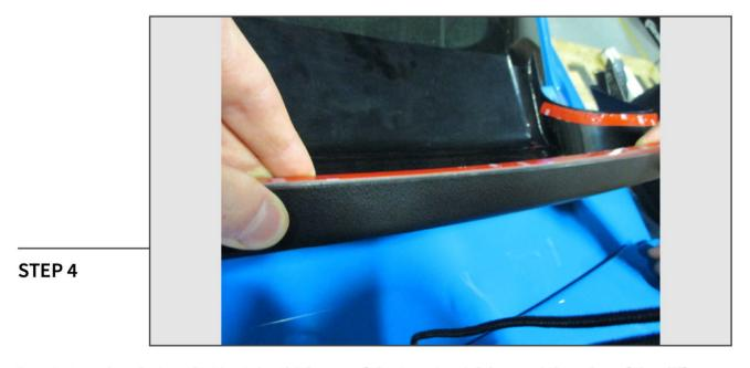
Locate tape bracket so that just the thickness of the tape is stick beyond the edge of the diffuser. Lightly contact the tape bracket to the diffuser until you're happy with the placement, then press firmly to seat the adhesive.
