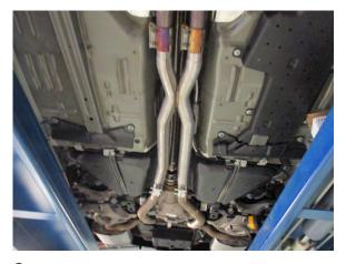
Step 5: Resecure the factory exhaust clamps onto the new resonator pipe.
