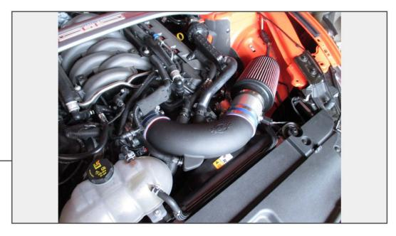
Install the assembled intake, making sure the intake tube sits flush against the throttle bottom opening. Reconnect the vacuum hoses and sound tube.
