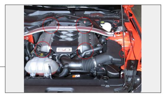
Remove the engine cover by firmly pulling the corners to pop the cover from the rubber mounts. Using a 10mm socket remove the bolt holding the air box to the inner fender.
