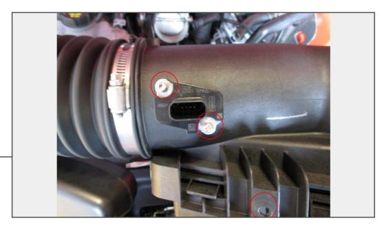
Using the supplied torx bit remove the mass air meter from the factory intake tube, you will not reuse the torx screws. The plug harness is attached to the air box, you must remove the wiring harness (bottom right of the picture) before you can remove the intake system. The system can be removed in one piece.
