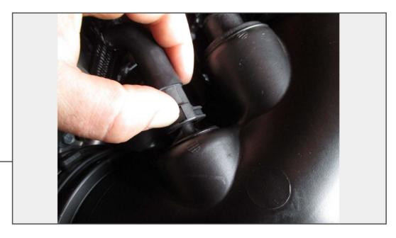
Pushing the dark section of the hose clamp will allow you to pull the vacuum line off the intake tube.
