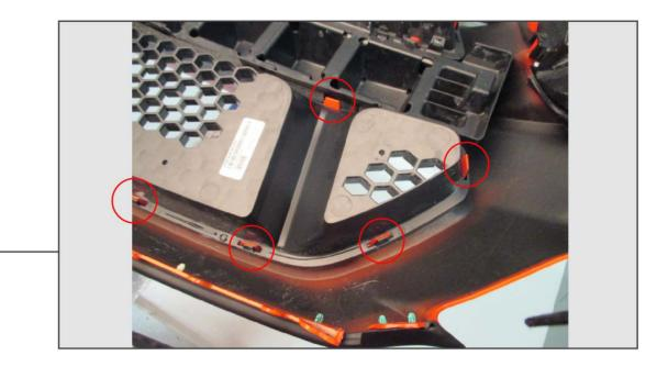
Using a large flat head screw driver, release the clips around the perimeter of the upper and lower grille. It's easiest if you start at the far left or right of the grille and work your way across.
