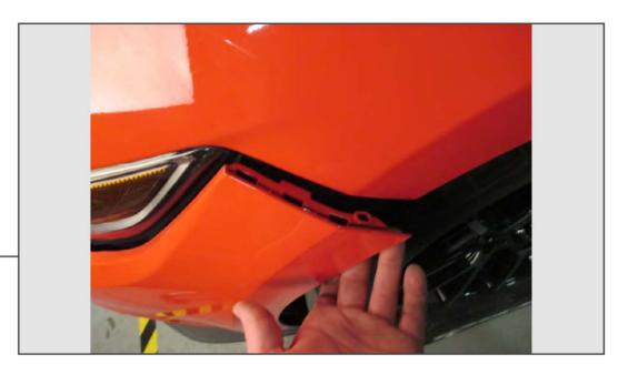
Once the bumper cover is ready to remove, using firm pressure pull the edge of the bumper to pop it from the clips. Have a helper support one side so that you don't scratch the paint. Slowly remove the bumper and support it on a soft non-abrasive surface.
