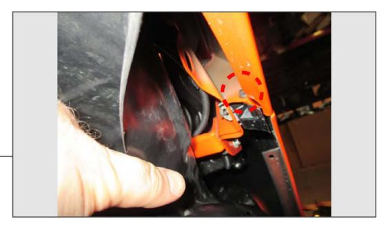
Fold back the fender liner so that you can access the (1) 8mm bolt that holds the bumper to the fender. It may help to remove the wheel for better access.
