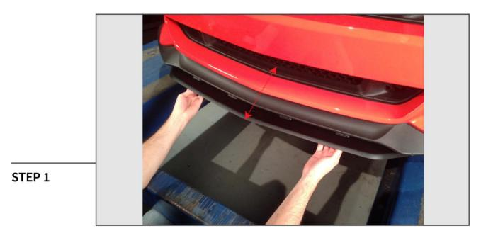
Raise and support the front of the vehicle. Center of the splitter with the center line of the bumper.
