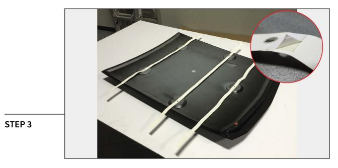
Remove the adhesive tabs on the supplied drilling templates, and stick them on the hood scoop. Each template is a different size, match them up with the appropriate mounting hole locations beforehand.
