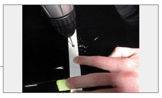
To prevent excess metal shaving from scratching the paint or falling into the engine bay, line the area around the hole with painters tape and lay a towel over the engine bay. Mark and drill a pilot hole on each of the (5) mounting locations. Once the pilot hole is drilled, drill a 9/32" hole through both the outer and inner layer of the hood. BE CAREFUL NOT TO DRILL TOO FAR, DAMAGE TO ENGINE COMPONENTS MAY OCCUR.
