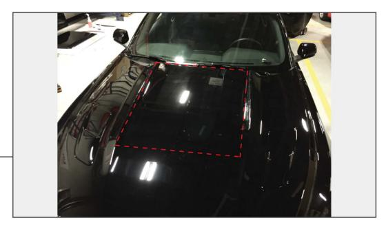
Using a supplied alcohol pad, clean the areas where the hood scoop tape will make contact with the hood. Once dry, treat the same areas with the supplied adhesion promoter. Let dry. Loosely install the hood scoop with the provided screws. Center the scoop side to side. Once you are happy with the placement peel the tape backing all the way off. Apply firm even pressure on the tape edges to ensure adhesion. Then tighten the hood scoop screws.
