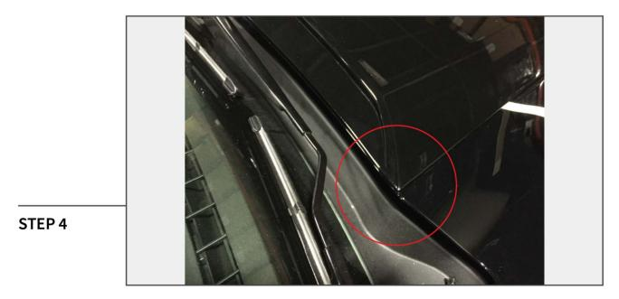
Place the hood scoop on the vehicle, line the back edge of the scoop up with the back edge of the hood and then center the hood scoop side to side.
