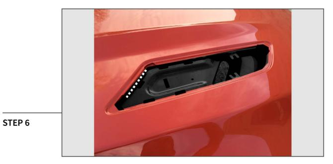
Apply downward pressure on the rear of the Vent so that the lip slides under the edge of the hood, then secure with the supplied washers and nuts. Repeat these steps for the opposite side.
