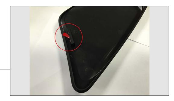
Test fit the Hood Vent Scoop so you have a clear idea of how it should fit. Then, remove the 3M tape backing from the mounting lip.
