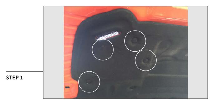
Remove the hood liner push pins and hold back the liner to gain access to the factory hood vent mounting nuts.
