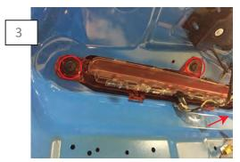
Unscrew the 3 plastic Phillips screws to remove the 3rd brake light.
