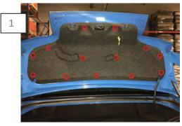
Begin by removing the deck lid liner, use a panel removal tool to remove the plastic clips.
