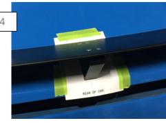
Loosely install the spoiler using the standard 4 mounting points. Align the supplied template with the base of the center most mounting bracket. Tape the edges of the template as seen above so that the template remains in place when the spoiler is removed. Then remove the spoiler.
