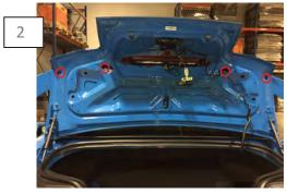
Remove the (4) factory spoiler fasteners and remove it from from car. \*\*Note: An extra set of hands is very helpful when removing the spoiler.
