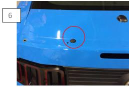
Install the provided plug by centering it over the deck lid hole, tighten the provided nut. Then install the spoiler using the provided hardware.
