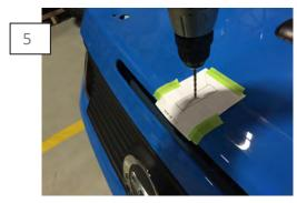
Using the template as a guide, drill a pilot hole, finishing with a 3/8 in" diameter hole. Remove any burrs using a file. \*\*Note: It is recommended that you apply paint to any bare metal around the hole to prevent corrosion.
