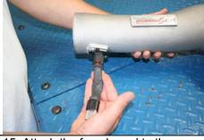
15. Attach the female end to the factory installed Mass Air Flow Sensor. Plug the side with the billet end into the engine harness. There is no need for additional brackets; the system was designed to support itself.
