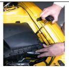
3. Remove the breather tube from both the stock air intake and the valve cover; you will no longer be using this piece.
