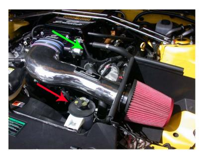
Note: In 2010 Model Mustangs, the power steering reservoir (pointed in red), is located in the area pointed to by the green arrow. All that needs to be done is to unbolt the power steering reservoir, and bolt it back onto the fan shroud, like in the picture.
