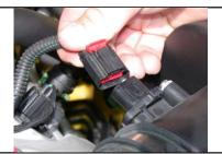
2. Sliding the red safety tab backward, unplug your factory mass airflow sensor. Depress the black and slide the connector from the sensor itself.
