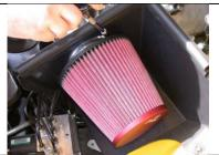
12. Place the air filter clamp over the air intake tube, followed by the air filter itself. Use the clamp to tighten the filter into place.
