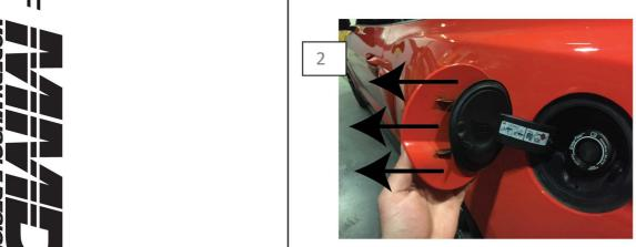
With the center clip upped up from step one, slide the factory fuel door off the fuel door hinge.
