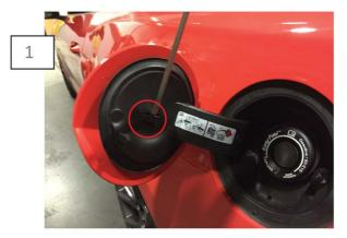
Open the factory fuel door. Using a small flat head screw driver, apply light pressure up on the center clip.
