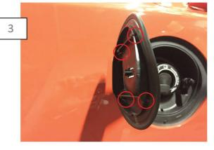
Line up the billet fuel door's (4) alignment tabs. Slide the fuel door onto the hinge until it clips.
