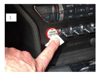
Begin by wiping down the dash panel surrounding the start button with the supplied alcohol wipe.
