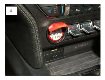
Firmly press the button cover onto the dash panel.
