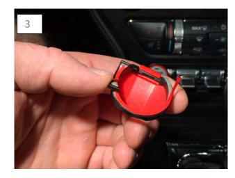
Peel off the tape backing.
