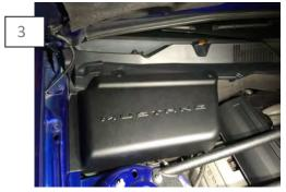
Position the part on the car so that the (2) mounting holes line up. Using the supplied push pins, install the battery cover. Then apply firm even pressure to the velcro to ensure proper adhesion.
