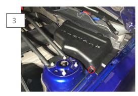
Position the part on the car so that the (2) mounting holes line up. Using the supplied push pins, install the battery cover. Place the hood latch cable in the notch. Then apply firm even pressure to the velcro to ensure proper adhesion.
