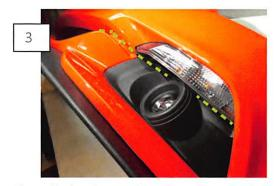
Thoroughly clean the mounting surface using soap and water (dashed lines above). Once dry, clean the surfaces with the provided alcohol wipe. Ensure the surface is completely dry.
