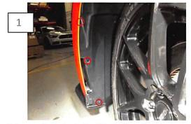
Gain access to the back side of the fog/turn signal bumper bracket. Raise the front of the vehicle using a jack and support with jack stands. Turn the wheels so that you can remove the clips holding the fender liner to the bumper.
