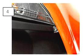
Before removing the tape test if the part so you can see how it fits the bumper. Apply slight pressure to the fog/turn signal bracket so that you can slide the bumper splitter between the bracket and the bumper.
