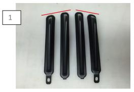
Arrange the Fins from left to right matching the picture above. The (2) on the left are for the driver side of the bumper. The (2) on the right are for the passenger side of the bumper.
