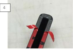
Remove the tape backing and apply adhesion promoter to the bumper. Allow time for the adhesion promoter to haze.
