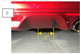
To locate the inner Fin, hook the inner Fin to the bottom edge of the bumper, then measure 5" from the center of the outer Fin to the center of the inner Fin. Repeat steps 3 and 4.
