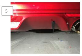
Then using the supplied push pin and mounting hole as a locator, align the Diffuser Fin so it looks straight from behind the vehicle and apply. Apply firm pressure to the Diffuser Fin and from behind the bumper to ensure proper adhesion.
