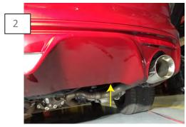
Clean the rear bumper of dirt and debris using soap and water, allow the paint to dry completely. Locate and remove the factory push pin.
