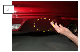
Wipe mounting location down with the supplied alcohol wipes circled above, allow the alcohol to haze.
