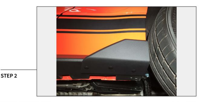
**REAR PLACEMENT:** With an extra set of hands, clamp, or painters tape, hold and carefully drill (3) 1/4" mounting holes in a staggered pattern. Please take caution when drilling, you only want to drill through the bottom surface of the chin spoiler. If you drill too far, you may drill through the top of the rocker panel. Secure the Winglet with the supplied push rivets.
