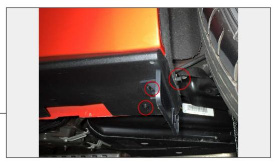
**REAR PLACEMENT:** Remove the (2) T20 Torx screws and (1) push clip attaching the rocker guard to the rocker. Locate the winglet by placing it against the rear edge of the rocker. Space the winglet 1/4" off the rocker panel, 1/4" gap is recommended, but the winglet can be moved in or out as desired. Use a clamp to hold the winglet in place so you can step back and confirm its placement.
