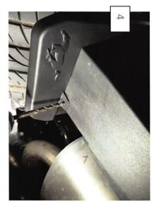
From below, drill the addition mounting location using a 1/4" drill bit. Mount using the supplied push clip.
