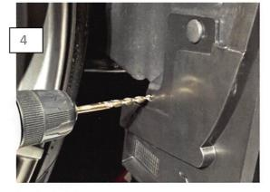
With the Splash Shield mounted, you can now drill the additional mounting holes. Begin by drilling a 1/4" hole through the Splash Shield into the fender liner. Install the supplied push clip.
