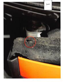
Raise and support the rear of the vehicle. Remove the factory splash shield retaining clip.
