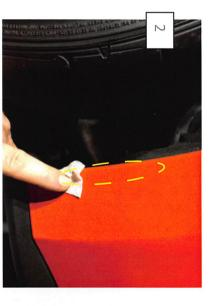
Clean the tape mounting surface with the supplied alcohol wipe. Allow time for the surface to dry. Then apply the supplied adhesion promoter and allow it to haze.
