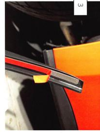
Remove the tape backing and mount the Splash Shield with the supplied push pin. Apply firm even pressure to the taped surface to ensure proper adhesion.
