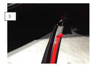
Peel off the tape backing. Position the Splash Shield and secure with the supplied push pin. Apply firm even pressure on the double sided tape to ensure proper adhesion.
