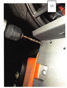
Now access the bottom of the rocker, drill the final mounting location with a 1/4" drill bit. Install the supplied push clip.
