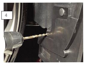
With the Splash Shield mounted, you can now drill the additional mounting holes. Begin by drilling a 1/4" hole through the Splash Shield into the fender liner. Install the supplied push clip.
