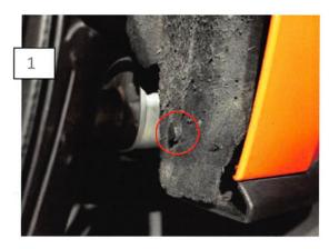
Raise and support the rear of the vehicle. Remove the factory splash shield retaining clip.
