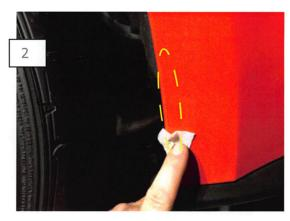
Clean the tape mounting surface with the supplied alcohol wipe. Allow time for the surface to dry. Then apply the supplied adhesion promoter and allow it to haze.
