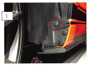
Raise and support the front of the vehicle. Turn wheel for better accessibility to the mounting locations. Begin by removing the factory push pin circled above.
