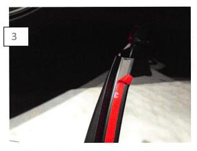
Peel off the tape backing. Position the Splash Shield and secure with the supplied push pin. Apply firm even pressure on the double sided tape to ensure proper adhesion.
