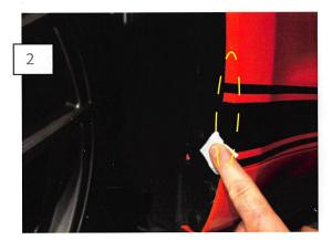
Using the supplied alcohol wipe clean the mounting location allow time for the surface to dry. Then apply the supplied adhesion promoter and allow it to haze.
