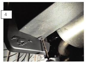
From below, drill the addition mounting location using a 1/4" drill bit. Mount using the supplied push clip.
