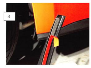
Remove the tape backing and mount the Splash Shield with the supplied push pin. Apply firm even pressure to the taped surface to ensure proper adhesion.
