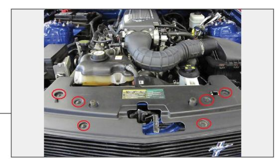
Remove the plastic radiator cover by removing the 6 plastic retaining clips.
