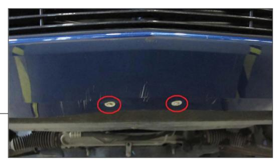
Remove the lower air deflector screws, along the bottom edge of the bumper, securing the bumper cover.
