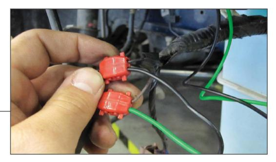
It is now time to wire your new headlights. You will be wiring them into the smaller 2- wire parking light bulb harness removed in Step 3. Use the scotch-locks provided to wire the headlights as follows.
