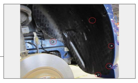
Begin by jacking the car up and removing the front wheels. This will make it easier to access the inner fender wells. Once the vehicle is properly supported, remove the three sheet metal screws and 5 plastic retainers holding the plastic inner fender well to the vehicle. Repeat for other side and remove inner fender wells
