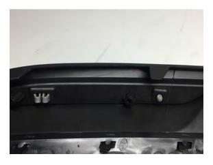
Step 19: Clip the bumper brace with the wiring harness to the new bumper. It will clip on using the factory center clip locations.
