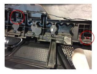
**Step 13:** Transfer the screw clips from the factory bumper over to the diffuser.
