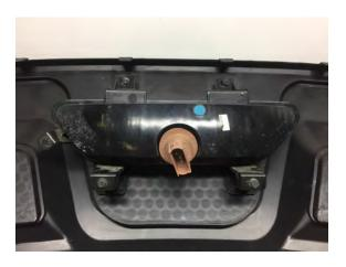
**Step 17:**If equipped with backup sensors, apply double-sided tape to the backup sensor brackets. Drill the hole for the backup sensors. There are marks in the bumper for where to drill and mount the brackets.
