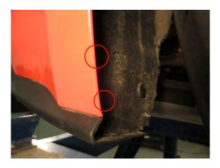
**Step 3:** Fold the fender liner out of the way to access the (3) bumper cover bracket bolts.
