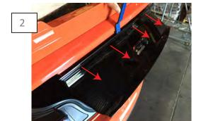
Use the panel removal tool to gently separate the factory deck lid panel from the deck lid.
