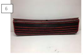
Apply the supplied tape to MP Concepts overlay, ensure all edges are covered. Remove the tape backing and install the overlay. Apply firm even pressure to ensure proper adhesion.
