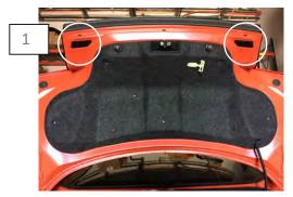
Using a panel removal tool, remove the caps covering the deck lid panel bolts. Then, remove the (4) 7mm screws.
