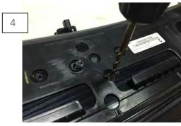
Remove the deck lid emblem by carefully removing the plastic weld from the back of the deck lid panel. Use an oversized drill bit and only remove enough material so that you can remove the emblem.
