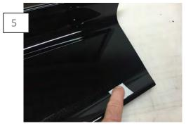
Wash the deck lid panel with soap and water. Allow the panel to dry. \*\*Recommended: Wipe the panel down with isopropyl alcohol to ensure the cleanest surface possible.
