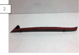
Prepare the fender vent by first installing the Fender Vent insert. Test fit the insert on the vent. Remove the insert and apply the supplied 3M double sided tape.
