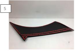
Install the 3M tape on the Fender vent as seen above. Before removing the tape backing, make yourself familiar with the way the vent fits on the vehicle.
