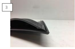
Test fit the insert again, ensure sure the end sit flush with the vent otherwise, the vent will not fit correctly on the car.
