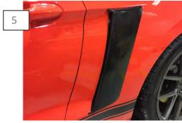
Test fit the scoop before removing the tape backing. Once you are comfortable with how the scoop fits, remove the tape backing. Apply firm even pressure to ensure proper adhesion.
