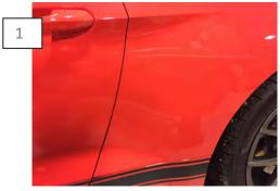
Wash the rear quarter panels with soap and water. Allow the panel and surrounding area to dry. \*\*Recommended: Wipe the panel down with isopropyl alcohol to ensure the cleanest surface possible.
