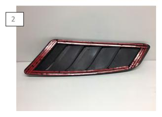
Apply the supplied 3M tape. Test fit the part on the hood to familiarize yourself with how the part should fit.
