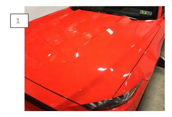
Wash the hood with soap and water. Allow the panel to dry. \*\*Recommended: Wipe the panel down with isopropyl alcohol to ensure the cleanest surface possible.
