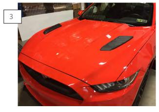
Measure from the front edge and side edge of the hood to ensure the louver is in the same place on both sides. Mark around the edges of the louver to ensures the louver is placed in the correct position. Remove the 3M tape backing and install. Apply firm even pressure to ensure proper adhesion.
