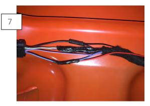
Splice the Red to the Blue/White wire on the reverse camera plug, and the Black wire to the Black wire on the reverse camera plug. Secure any excess wiring to the factory wiring harness using cable ties.
