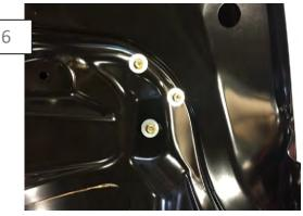
Thread the supplied studs into the spoiler leaving only enough thread exposed on the underside of the decklid to install the supplied washer and nut. \*\*Note: Do not over tighten these nuts. Doing so can cause damage to the decklid.
