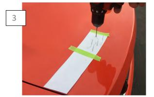
Carefully pre-drill the spoiler holes using a 1/8" drill bit. You will need to drill straight through the outer and inner deck lid panels. Finish drilling the holes to 11/32". Optional Brake: drill an additional 1/4" hole on the passenger side for wiring. \*\*Note: Apply touch up paint to any exposed metal to prevent oxidation.
