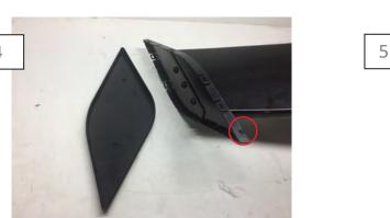
Attach the spoiler extensions to the spoiler using the provided Phillips screws. Once the extensions are installed, press on the end caps. \*\*Note: The opening circled above will be on the top side of the spoiler.
