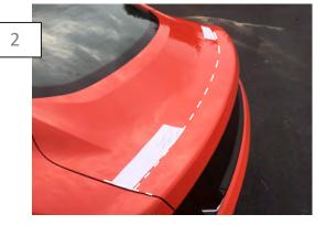
Align the left and right drill templates along the deck lid body line and the outside edge.
