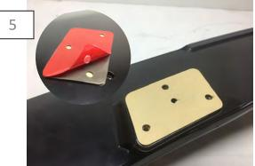
Apply the double sided tape pads to the bottom of the spoiler. Thoroughly clean the spoiler mounting locations prior to installing the spoiler to ensure proper adhesion. Test fit the spoiler to ensure all the holes line up prior to removing the red tap backing.
