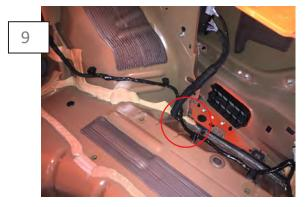
Carefully remove the factory electrical tape to gain access to the wires.
