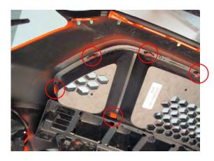
**Step 11:**Using firm pressure, clip the Shark Bite Grille into the bumper cover using the factory tabs. \*\*Note: Ensure the grille "clicks" onto all the tabs.
