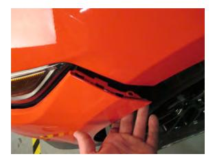
**Step 9:**Begin by removing the plastic bumper brace. Gently bend tabs as needed to remove support.
