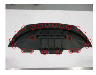
**Step 5:**On each side of the bumper, remove the (3) plastic clips holding the fender liner to the bumper.
