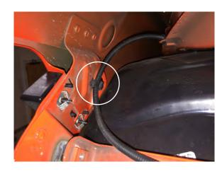
**Step 17:**Remove the (1) 10mm bolt securing the fender to the vehicle.
