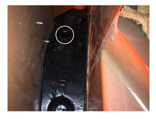
**Step 19:** Once the foam is removed, remove the (2) 10mm bolts securing the fender to the vehicle.
