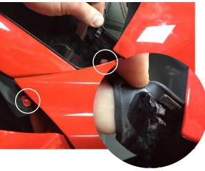
**Step 21:** Remove the (3) 10mm bolts securing the fender to the vehicle. At this point the fender will be ready to remove from the vehicle.
