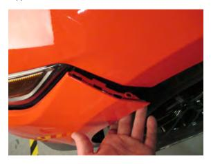
**Step 9:** Remove the (3) push clips holding the inner fender liner to the rocker panel.
