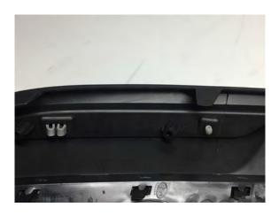
Step 11: Reinstall the diffuser to the bumper in the reverse order.
