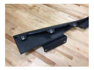
**Step 10:** Transfer the reflectors from the factory bumper to the new bumper. They are held on with a 10mm nut.
