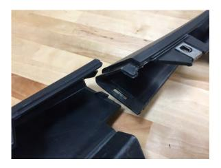
Step 9: Transfer the screw clips from the factory diffuser trim panel to the new diffuser.
