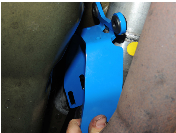
FIG 4 – Upper Bracket installed sideways
