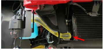
110. Insert the LTR to Manifold hose through the hole on the upper shroud and secure to the top LTR bung with a hose clamp from Bag # 3. Secure the other end to the lower bung on the supercharger manifold.
