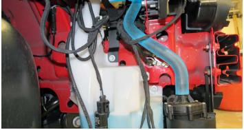
113. Secure the Surge Tank to Manifold hose to the surge tank and manifold using two (2) hose clamps from Bag # 3.
