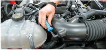
40. Disconnect the brake aspirator hose from the manifold PCV hose.
