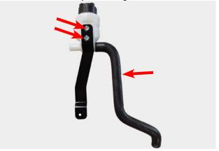
112. Connect the Water pump to Surge tank hose to the water pump and secure with a hose clamp from Bag # 3.
