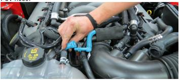
41. Using a flathead screwdriver, loosen two (2) worm clamps securing the air inlet tube and remove.
