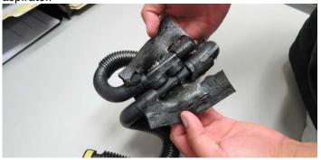
97. Remove the hose that attaches to the check valve and replace with the supplied 3/8" hose. Attach the supplied vacuum cap to the opposite end of the aspirator.
