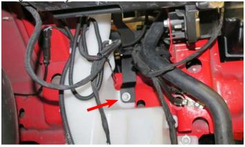
115. Using a razor blade, or equivalent, remove the  $90^{\circ}$  quick connect fitting on the factory passenger side PCV hose.
