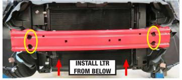
104. Install the supplied beams using the two (2) M8 x 30mm hex flange bolts from Bag # 3, loosely screw in the bolts through the crash beam braces. The lower crash beam braces will sandwich the LTR to the crash beam and be secured using the M8 nuts and washers supplied in Bag # 3. Once all bolts are in place through the braces, fully tighten the bolts and nuts.
