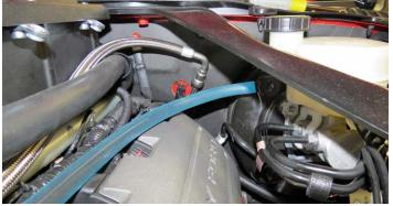
100. Route the Aspirator to Manifold hose under the heater hose and attach to the fitting on the supercharger nose.
