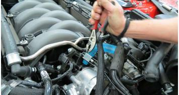
46. Remove the brake aspirator hose assembly from the brake booster and set aside as it will be reused later.
