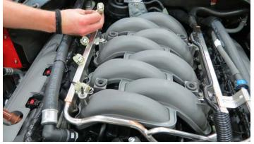
53. Place a rag underneath the fuel input line. Lift up the blue locking tab and disconnect the fuel line from the rail and from the hard line on the firewall.
