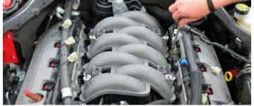
56. With the manifold bolts removed, carefully position the manifold forward and remove four (4) sensor connectors and two (2) harness clips.
