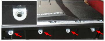
76. For proper bracket alignment, test fit the side covers onto the brackets using eight (8) M6 X 25mm bolts from the side cover kit. While pushing the side covers forward, fully tighten the bracket bolts. Once all brackets are aligned and tightened, remove the side covers.
