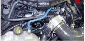
96. Carefully remove the protective foam from the brake aspirator.
