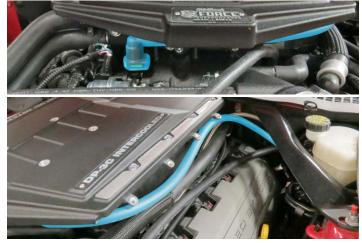
119. Connect the supplied straight quick connect fitting on the EVAP hose to the hard line.
