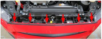
26. Using a 5.5mm socket, remove two (2) bolts under the weather stripping, one per side.
