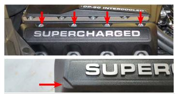
WARNING: Launching the vehicle may cause wheel hop which will induce engine torquing. The engine movement may cause the passenger side coil/side cover to make contact with the strut brace. Available aftermarket Wheel Hop Eliminator kits should be considered if this problem occurs. Additional clearance may be required to alleviate any contact in the strut brace area.
