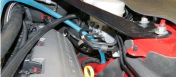
120. Zip tie the Fuse holder on the Water Pump/EVAP Harness onto the top right corner of the fuse box.
