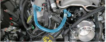
49. Disconnect the throttle body connector.
