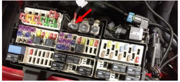
122. Route the "Intercooler Water Pump" end of the Water Pump/EVAP Harness below the fuse box and around the washer fluid reservoir and plug it into the intercooler water pump.
