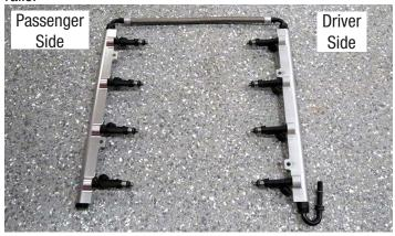
80. Apply O-ring lube to both ends of the supplied fuel injectors, then install them into the supplied fuel rails, oriented so the electrical connectors will face away from the supercharger.
