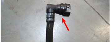
116. Attach the  $90^{\circ}$  fitting onto the supplied  $1/2^{\circ}$  Cadbar hose. Connect the quick connect fitting to the passenger side valve cover and the other end of the hose to the barb on the supercharger nose.
