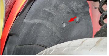
30. Remove two (2) bolts, one per side, securing the fascia to the fender using a 7mm socket.
