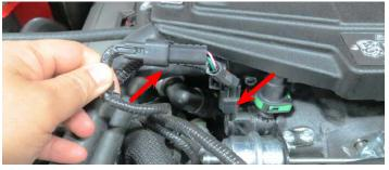
125. Installed the provided throttle body and adaptor plate using the four (4) M6 x 55mm bolts located in bag #5 and two (2) O-ring gaskets (one on each side of the spacer). The four (4) M5 bolt holes will not be used and are intended for mounting the GT350 87mm throttle body.
