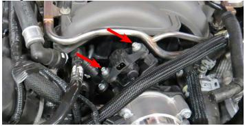
78. Install the EVAP solenoid to the supercharger manifold using two (2) M6 x 25mm bolts in Bag # 1.
