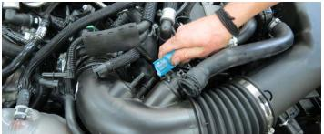
39. Remove the additional brake aspirator hose from the air inlet tube.
