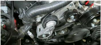
68. Using the M8 x 20mm bolts and M8 washers supplied in Bag # 2, install two idler pulleys to the tensioner bracket. The top idler pulley is 65mm and the lower idler is 76mm. Add a small amount of blue thread lock fluid to the threads ONLY, do not allow excess thread lock fluid to drip onto the pulley's bearings. Torque the bolts to 18 ft-lbs.
