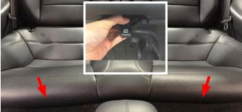
2. Remove the rubber access plug on the drive side and disconnect the fuel pump electrical connector.
