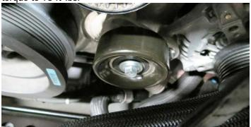
67. Verify that the tensioner is clocked correctly by sliding the index through the hole on the bracket. Install the supplied belt around the tensioner pulley and torque the M10 bolt supplied in Bag # 2 with a 15mm socket to 32 ft-lbs.
