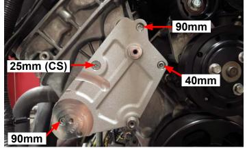
63. Using a 13mm socket, remove the factory tensioner adjacent to the alternator and balancer.
