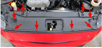
25. Remove six (6) bolts securing the top of the fascia using an 8mm socket.
