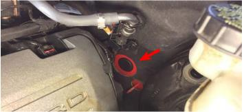
48. Remove the passenger side PCV hose from the valve cover and the intake manifold.
