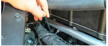
88. Reconnect the injector connectors to the appropriate fuel injectors. *WARNING: Never attempt to rotate the injectors*.
