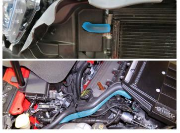
111. Attach the surge tank bracket to the surge tank using two (2) M6 x 10mm bolts from Hardware Bag # 3. Also attach the water pump hose to the surge tank and secure it with a hose clamp from Bag #3.
