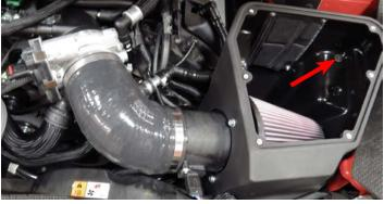
131. Install the conical air filter onto the MAF housing inlet using the provided clamp.
