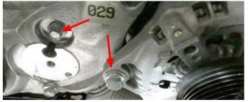
65. Secure the idler bracket by installing bolts from Bag # 2. The M10 x 110mm bolt through the ear of the alternator, the M8 x 90mm bolt into the top front cover hole, and the M10 x 45mm bolt through the lower hole that was used to secure the stock tensioner. Use blue thread lock fluid on all of the bolt threads and torque all bolts to 22 ft-lbs.
