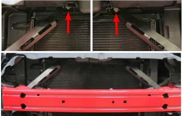
105. Using a drill and a 1 1/4" hole saw bit, drill a hole in the shroud that lines up vertically and parallel with the lower LTR barb.
