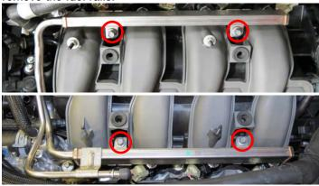
55. Using an 8mm socket, remove six (6) manifold bolts.
