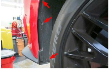
29. There is an additional push pin located just above the tire that needs to be removed.
