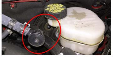
47. Remove the sound generator assembly and plug the hole in the firewall using the supplied plastic grommet plug supplied in Bag # 1.
