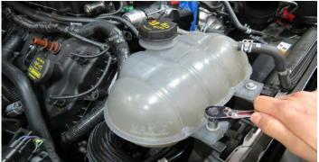
95. Install the supplied coolant bleed hose and secure with the factory hose clamps.
