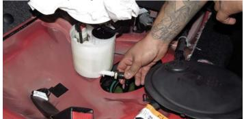
19. Remove the OEM fuel pump module from the vehicle being careful not to spill any fuel.
