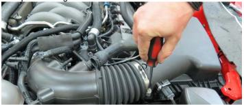
42. Disconnect the MAF sensor harness by pulling back the red locking tab and depressing the locking clip.
