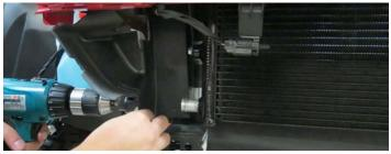
106. Using a drill and a 1 1/4" hole saw bit, drill a hole in the shroud that lines up vertically and parallel with the upper LTR barb. *CAUTION: Be mindful of the A/C hard lines behind the shroud.*
