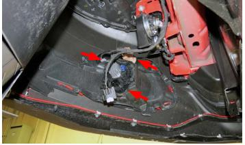
32. Tape up the fender as needed to prevent scratching the painted surfaces. With the help from an assistant, carefully disengage both sides of the fascia by gently pulling the sides outwards. Remove the fascia and set aside.
