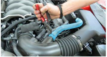
37. Remove the brake aspirator hose from the air inlet tube.
