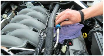
54. Using a 10mm socket, remove four (4) bolts securing the fuel rail and manifold. *TIP: It's not required to fully remove the fuel rails.*
