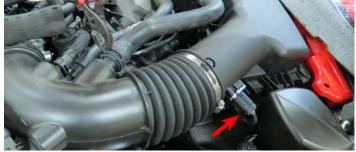
43. Make sure the MAF harness is free from the lower air box. Then, remove the factory air box bolt and remove the air box from the vehicle. Save the bolt.
