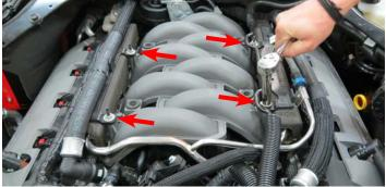
51. Remove the retaining brackets and the foam insulators from the fuel rails.
