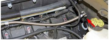
91. Reinstall the passenger side heater hose fitting using the factory hardware.
