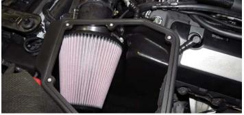
132. Install the air box lid using the six (6) 1/4"-20 cap screws and washers located in bag #5.
