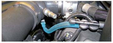
134. Connect the  $90^{\circ}$  fitting on the supplied driver side PCV hose to the driver side valve cover. Connect the other end to the fitting on the silicone elbow.
