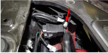
124. Connect the factory EVAP connector onto the "Engine Harness" end of the "Water Pump/EVAP Harness" and the "EVAP Solenoid" end onto the EVAP solenoid.
