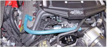
117. Using a razor blade, remove the  $90^\circ$  fitting on the factory EVAP hose.
