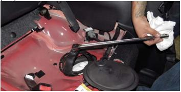
18. Carefully lift the fuel pump module out of the tank and disconnect the crossover line by depressing the yellow locking tab and pulling the line off of the fitting.
