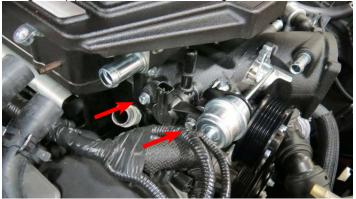
79. Using O-ring lube, install the fuel rail fittings onto the fuel rails. The passenger side rail will have the black plug on the front of the rail, while the driver will have the 180° fitting. Attach the supplied fuel crossover to the rear of both rails.
