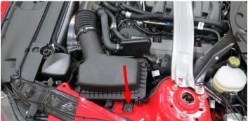
44. Disconnect the EVAP connectors and fully remove the EVAP hose .
