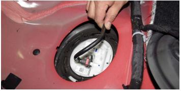
**NOTE:** Prior to removing the fuel pump module, remove any dirt or debris around the fuel tank opening with compressed air or shop vac.
