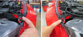
27. Remove sixteen (16) bolts and six (6) push pins securing the splash guard using a 7mm socket and a panel puller. Remove the splash guard and set aside.
