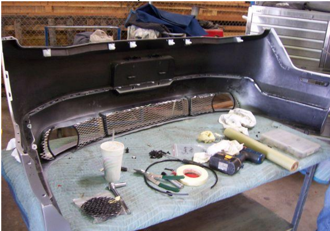
You can see the white Clips where the top snaps into place.
