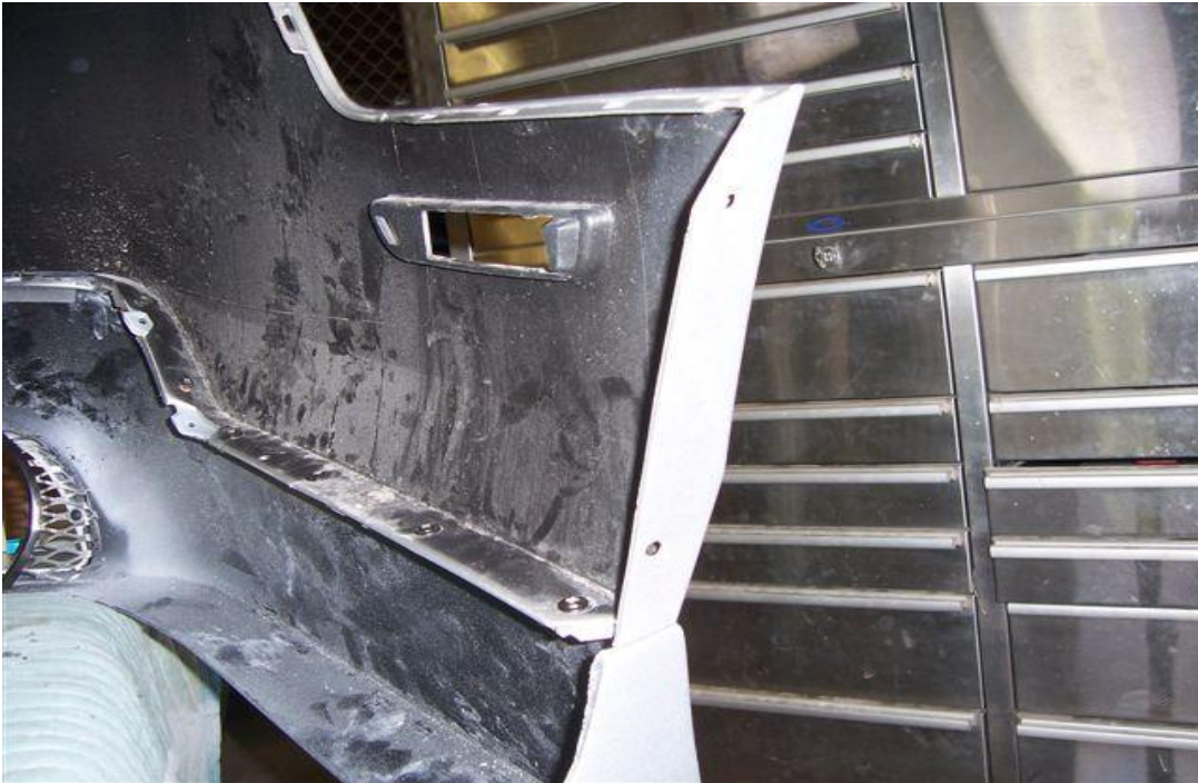
About Four Bolts hold each side into place.
