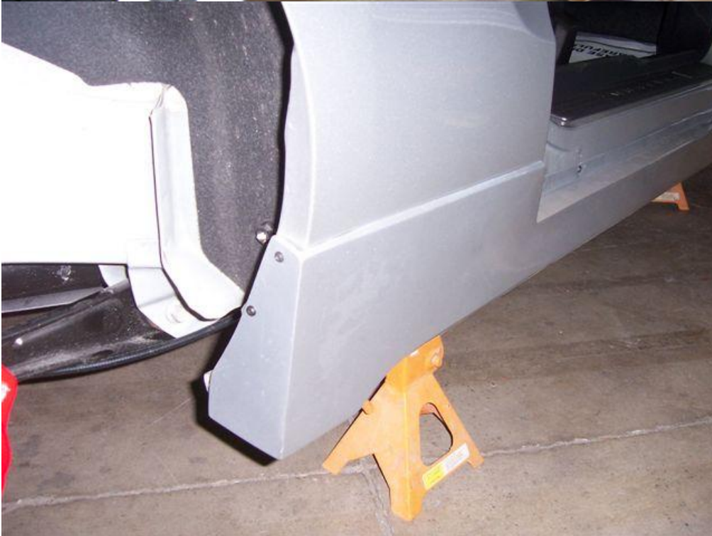
Two Screws on each side on the fender wells, self tap screws work okay here, but you can make a pilot hole if you want too.
