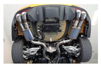
**Step 5.** Finish the initial installation by fitting the Muffler Assemblies onto the Mid pipe Assemblies using the supplied 3.00" clamps and inserting the hangers into the rubber insulators.
