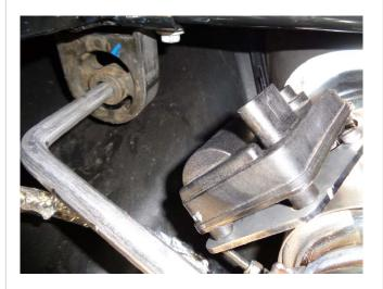
**Step 6.** If your vehicle has valves re-connect the wiring harness plugs to the Valve motors.
