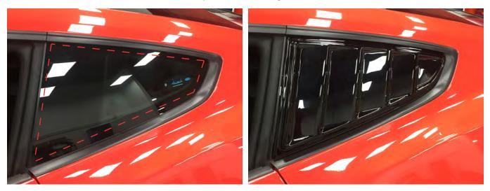
**Step 3**// Once you are comfortable with where the parts mount remove the tape backing. Apply the supplied adhesion promoter to the tape surface then install the louver to the vehicle.
