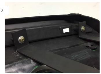
Secure the Quad Tips to the upper mounting locations using the provided screws. **\*\***Note: Do not over tighten the screws. Doing so can pull the threads out of the bosses.
