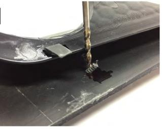
Using scribe, mark the locations of the lower mounting holes. Remove the Quad Tips and drill the scribed holes to
