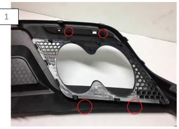
Begin by locating the mounting locations for the Quad Tips. The upper (2) mounts are screw bosses. The bottom (2) mounting locations will need to be marked and drilled.
