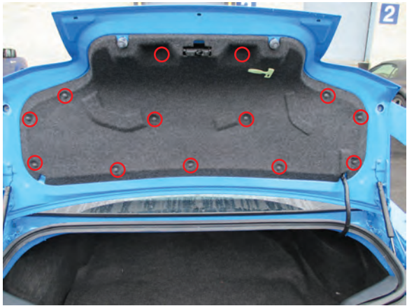
Step 1 Open the trunk and remove the various push pins securing the trunk lid panel to the trunk.
