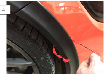
Hold the flares in place. With the flare in position, peel the tape backing as you lightly apply pressure to hold the flare in place. Once the tape backing is fully removed, apply firm even pressure to the tape surfaces to ensure proper adhesion.
