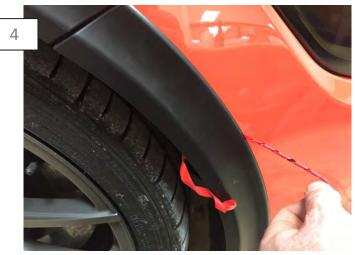
Hold the flares in place. With the flare in position, peel the tape backing as you lightly apply pressure to hold the flare in place. Once the tape backing is fully removed, apply firm even pressure to the tape surfaces to ensure proper adhesion.
