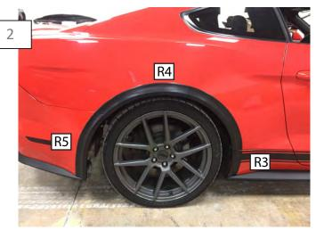
Before installing the flares, test fit the flares to familiarize yourself with where they fit best. \*\*Note the back of the parts are labeled R3, R4, and R5 for the right side. L3, L4, and L5 for the left side.
