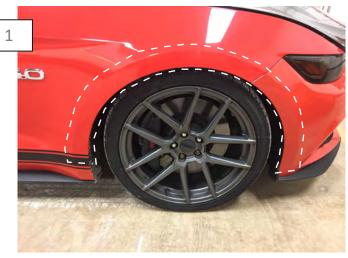
Begin by throughly cleaning the front fenders and inner fender lip with soap and water. Allow time for the bumper to dry. Using isopropyl alcohol to remove any wax or grease is highly recommended. Apply the isopropyl alcohol to a clean tint free cloth and wipe the paint surface.
