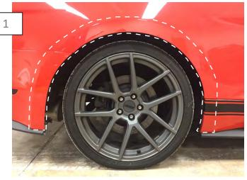
Begin by throughly cleaning the Rear fenders and inner fender lip with soap and water. Allow time for the bumper to dry. Using isopropyl alcohol to remove any wax or grease is highly recommended. Apply the isopropyl alcohol to a clean tint free cloth and wipe the paint surface.
