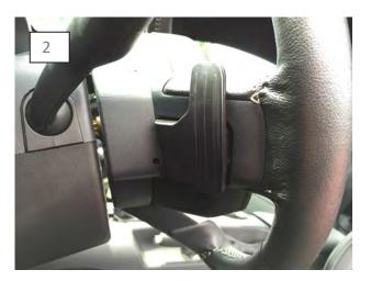
Clean the mounting surfaces with the supplied alcohol, allow time to flash dry.
