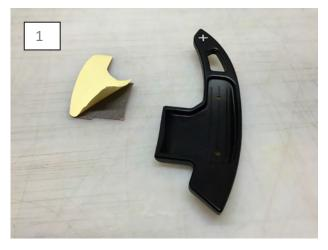
Clean the paddle extension with the supplied alcohol wipe allow time to flash dry Then peel back the adhesive backing and apply the double sided tape to paddle extension.
