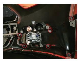
**Step 7**Using a 7mm socket, remove the screws holding the turn signal bracket to the bumper. Use a flat head screwdriver to assist in releasing the clips.
