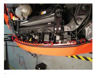
**Step 2**Remove the (8) bolts securing the bumper cover to the radiator support.
