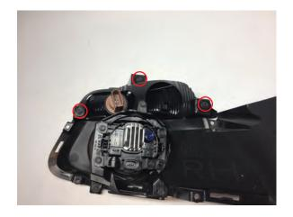
**Step 8**Remove the (3) 7mm screws holding the turn signal to the bracket. Then remove the turn signal.
