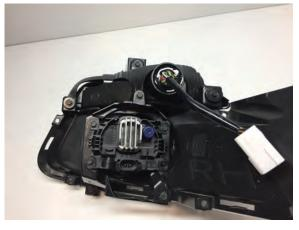
**Step 9**Using the existing hardware, reinstall the Smoked LED Turn Signal. \*\*Note: Be careful not to pinch any wires. Reinstall in reverse order.
