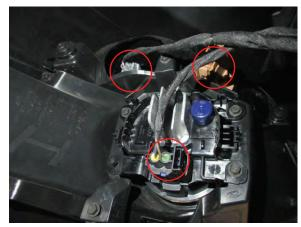
**Step 6**With the splash shield pulled back, you can access the plugs for the turn signals and fog lights. Then remove bumper.
