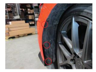
**Step 4**On each side of the bumper, remove the plastic clips holding the fender liner to the bumper.
