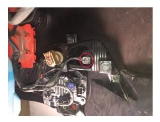
**Step 7**Feed wiring safely across the top of the inner splash shield to the front of the vehicle. Using a panel removal tool, remove the front section of the front fender (3) splash shield clips. With the splash shield pulled back, locate the side market light socket.
