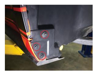
**Step 6**Using a panel removal tool, locate and remove the rear section of the front fender (3) splash shield clips. Gently pull splash shield back to gain access to the emblem wiring.
