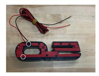
**Step 3**Apply the supplied 3M tape to the back of the LED emblem as shown. \*\*Note: Be sure not to cover the holes where the wiring comes out, and the ventilation hole.
