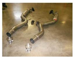
1) Place the new Flowmaster muffler assemblies next to the factory units and swap the front and rear hanger mounts from the stock mufflers to the Flowmaster assemblies. Also, place a provided 2.25" clamp onto the inlet of each assembly. Tighten the clamp just enough to hold in place.
