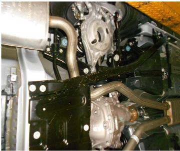
2) On convertible model vehicles, the body braces shown in the photos above will need to be removed in order remove the factory system and install the Flowmaster system. Starting at the front of the right side (passenger) brace, loosen the front bolt and then work your way to the rear of the vehicle removing the next eight bolts, lower the brace from the vehicle. Repeat this step on the left side of the vehicle with the six bolts on that side.
