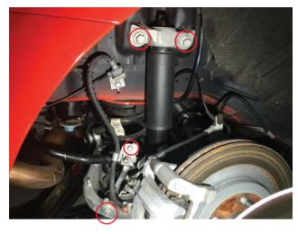
**Step 3:** Remove the lower (2) shock mount bolts from the lower control arm, remove the shock from the vehicle.
