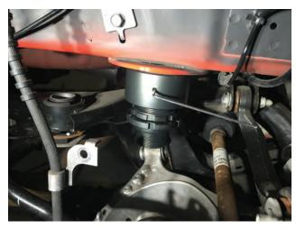
**Step 9:** Place the plastic spring isolator on top of the spring.
