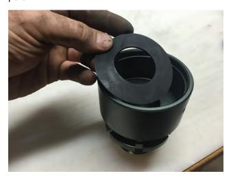
**Step 8:** Install the upper spring perch, use the allen set screw to hold the perch in place.
