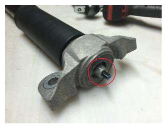
**Step 12:** Reinstall the upper mount on the SR shock, reinstall factory plastic cap.
