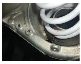
**Step 11:**Raise the rear subframe with the jack and slowly tighten the (4) rear subframe bolts to 129 ft/lbs. Then re-tighten the (4) front subframe brace bolts to 41 ft/lbs.
