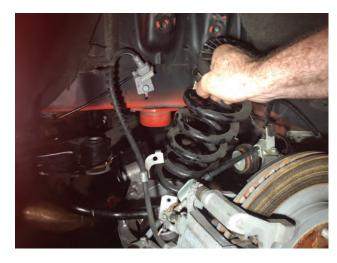
**Step 7:** Place the supplied rubber isolator in the upper spring perch.
