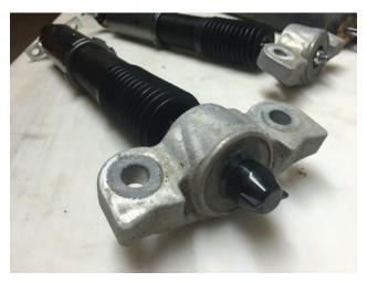
**Step 13:**Lengthen the shock body by unscrewing the lower shock mount until the shock is long enough to bolt on. Install the shock using the factory bolts and provided lock nuts..
