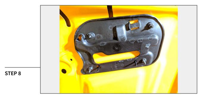
Remove the backing from the tape on the hood vent. Insert the hood vent into the hood, and secure using the factory (4) nuts. Press firmly on the taped area to fully seat the adhesive.
