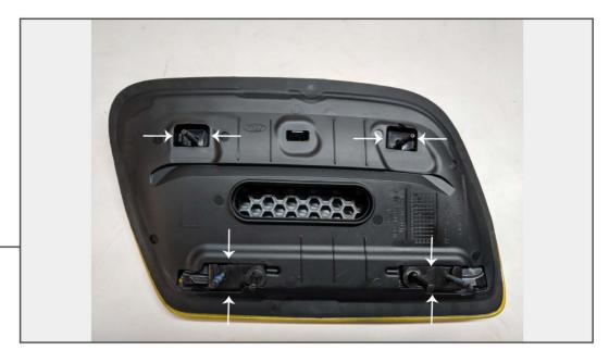
Using a flat head screw driver, remove the inner vent cover from the factory vent by releasing the plastic tabs in the locations shown above.
