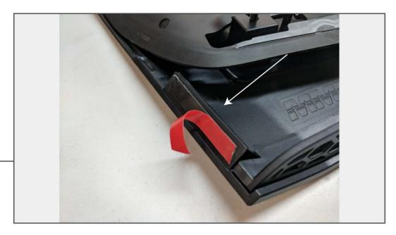
Using the supplied alcohol pads, clean the area where the tape will make contact with the hood surface.
