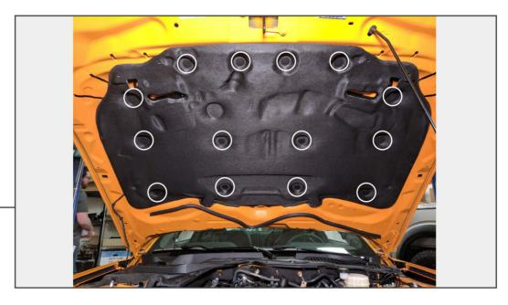
Begin by thoroughly cleaning the hood of your vehicle with automotive soap and water. Next, remove the inner hood liner push rivets to remove the liner and gain access to the hood vent.
