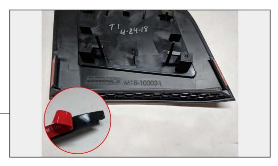
Remove the tape backing on the honeycomb insert. Make sure the corners of the insert sit flush with the edge of the hood vent and do not stick above. Once you have the insert lightly in place, press firmly to fully seat the adhesive.
